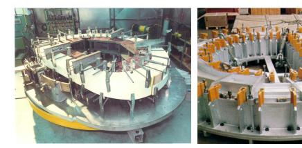
Turns assembly on winding table
